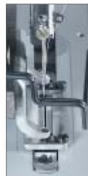
Position of the needle bar during sewing
