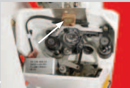
+ Functional bobbin thread monitor with rest thread sensor -926/06 (optional)
